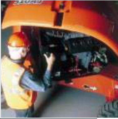
Swing out engine for ease of service
